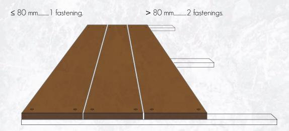
The battens are fitted perpendicular to the panels and must be properly protected against corrosion and rust, independently of the material or system used.
