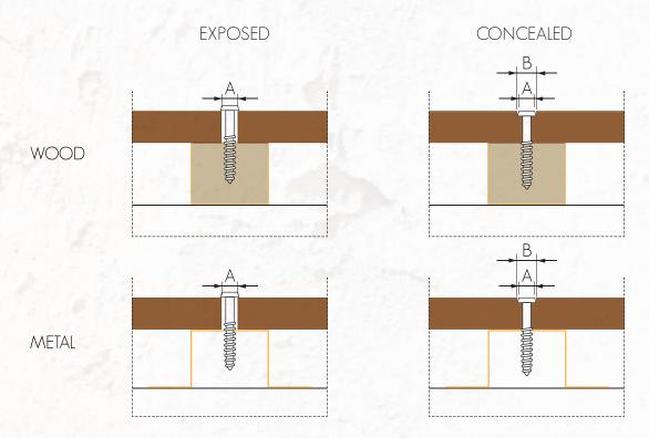
It is particularly important to ensure that the screw is exactly centred in the hales.
