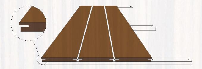
The battens are fitted perpendicular to the panels and must be properly protected against corrosion and rust, independently of the material or system used.
