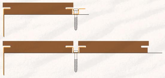
The next machined panel is then slotted into the other side of the staple:
